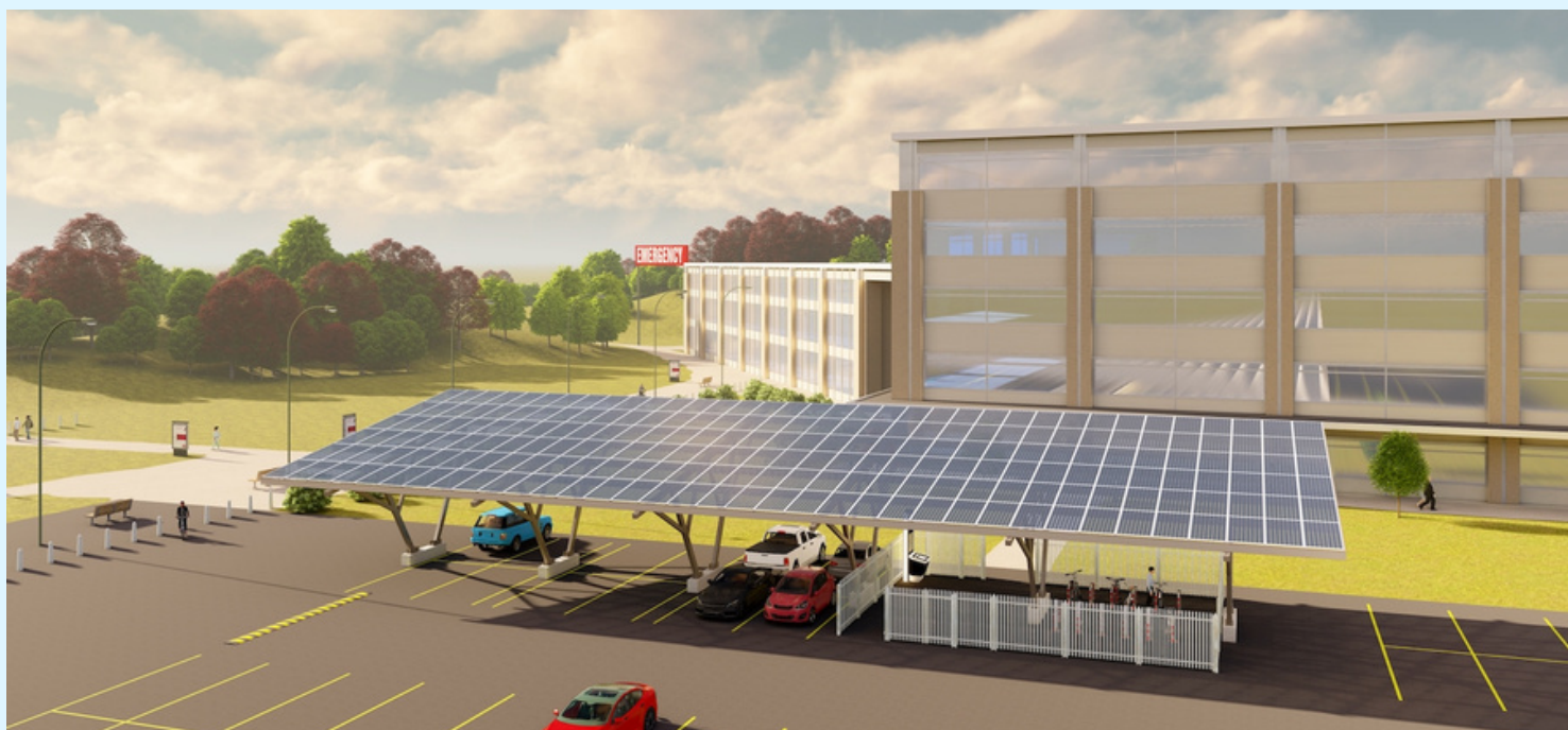
Sloping solar canopies elegantly combine vehicle shelter and power generation, providing rain and snow management that goes beyond just power generation. Note covered outdoor e-bike/BPMM charging feature. SOURCE: VCT Group https://vctgroup.com
